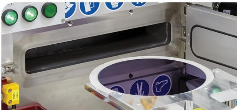
Manual device for loading and unloading of 200 mm wafers. The system is prepared to fit into a cluster system with a central transfer robot module, load locks and further process modules.
